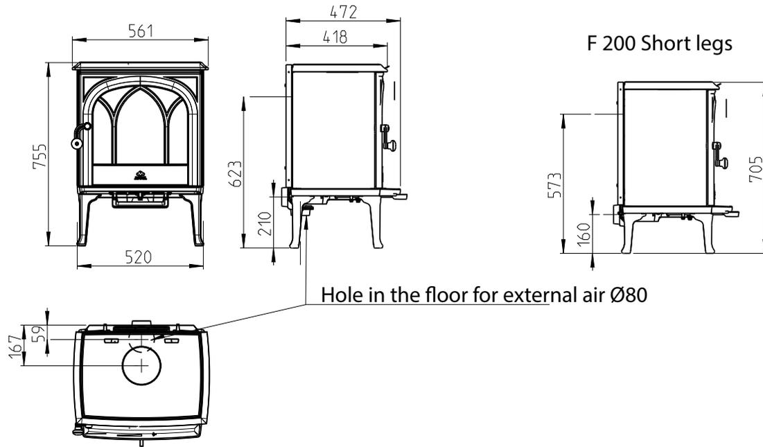
Hole in the floor for external air Ø80
