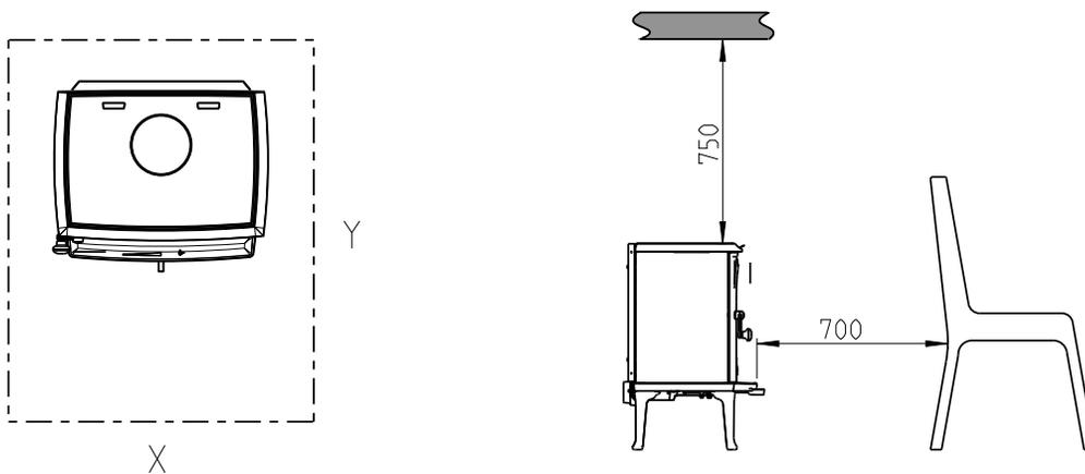
Min. measurements floor plate
